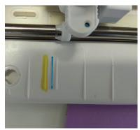
Mount printed or bare cardstock onto the Silhouette Portrait 2 cut mat by placing the project onto the sticky surface so that the top-left corner is aligned with the marks on the cut mat labeled 8½" x 11" (see image above). Feed the cut mat into the Silhouette Portrait 2 and 3 by aligning the left edge of the cardstock (not the cut mat) to the center line of the group of short lines on the left side of the feed area. Press the **Up Arrow** button on the Silhouette Portrait 2 and 3.
