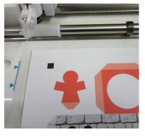
Click **Send to Cutter** to begin fabricating your project. The Silhouette digital fabricator will scan and detect the registration marks if the option is selected, and proceed to cut the paper. When the cut process has completed, the Silhouette digital fabricator will eject the cut mat. Press the **Unload** button or down arrow on the cutter to release the cut mat completely. Carefully peel the cut cardstock off of the cut mat.
